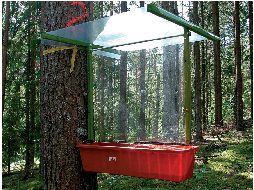
Fig. 2. Trunk window trap, designed by I. Süda in 2004 (photo by I. Süda).
