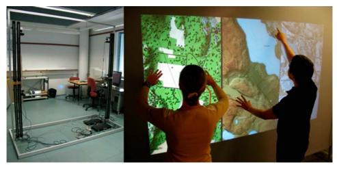
*Figure 2.* Our original rear projection setup for the multi-touch system, with a projector, computer, IR cameras and IR lights at the back (on the left) and a large canvas on the front displaying the map application (on the right).
