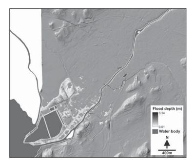
**Figure 7.** A flood inundation map based on the LiDAR DTM (1m grid). The flat, high-level areas mid- and upstream prevented the correct merging of the modelled water surface elevation to the topography (Note, islands in the river were not mapped and "flood ponds" were not removed from the inundated area).
