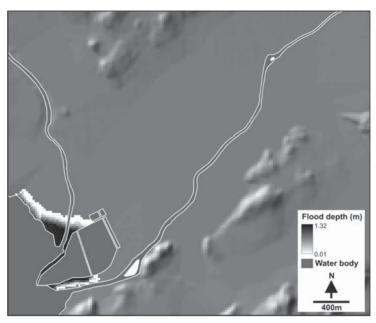
**Figure 5.** A flood inundation map based on the 25 m DTM. The flat, high level areas in the mid- and upstream reaches prevented the correct merging of the modelled water surface elevation with the topography. The waste management plant is located nearby on the square-type water body (Note, islands in the river were not mapped).
