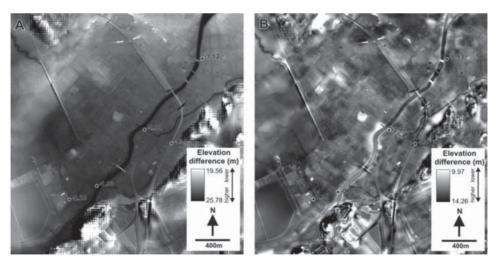
**Figure 3A-B.** Difference images of the LiDAR DTM vs. 25 m DTM (A) and LiDAR DTM vs. 10 m DTM (B). The difference images were processed without bathymetric data. The black dots with elevation values (m) on both images represent elevation differences between LiDAR DTM and 25 m DTM (A) and LiDAR DTM and 10 m DTM (B). See table 2 for further statistics of the DTM comparisons.
