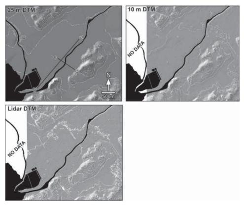
*Figure 2.* Hillshade visualisation of the DTM's used in this study (25m DTM; 10 m DTM; Lidar DTM). The 5 m contours were visualised on the all three DTM's. Location of the elevation profile is shown on the 25 m DTM.
