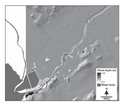
**Figure 6.** A flood inundation map based on the 10 m DTM. The flat, high-level areas midand upstream did not allow for the correct merging of the modelled water surface elevation to the topography (Note, islands in the river were not mapped and "flood ponds" were not removed from the inundated area).
