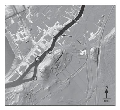
**Figure 8.** A subset of the LiDAR DTM flood inundation map along the downstream section. The damming effects of the embankments and flood water on the dykes were easily recognised. Flood water ponds and their possible connection to the river could also be analysed. Some erroneous riverbanks are highlighted with black circles.
