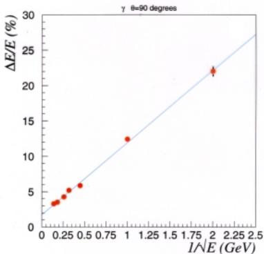
Resolution obtained as a function of  $\mathbf{E}_{\gamma}$   $\Delta E/E = (10.3 \pm 0.3)\% / \sqrt{E} + (1.1 \pm 0.1)\%$
