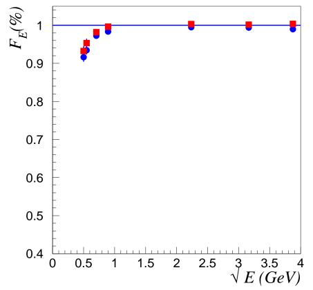
Fraction of collected energy is never less than 92% even when only the most energetic cluster is taken into account
