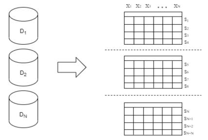
Figure 2. Horizontal data partitioning with each data shard sharing the same feature space.
