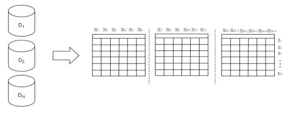
Figure 3. Vertical data partitioning with each data shard sharing the same sample space
