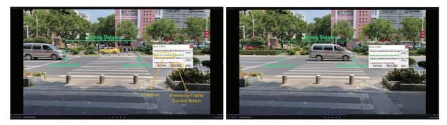
Figure 4 – The speed extraction process for vehicles by using the KMplayer software
