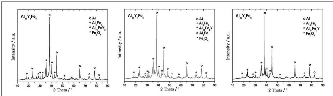
**Figure 1** XRD patterns of  $\text{Al}_{88}\text{Y}_6\text{Fe}_6$ ,  $\text{Al}_{88}\text{Y}_7\text{Fe}_5$ , and  $\text{Al}_{88}\text{Y}_8\text{Fe}_4$  alloys in the form of plates in as-cast states
