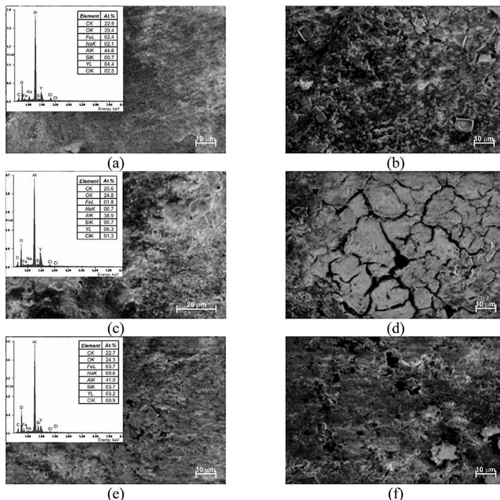
Figure 3 SEM images and EDS analysis of the surface morphology of  $\text{Al}_{88}\text{Y}_8\text{Fe}_4$  (a, b),  $\text{Al}_{88}\text{Y}_7\text{Fe}_5$  (c, d), and  $\text{Al}_{88}\text{Y}_6\text{Fe}_6$  (e, f) alloys in the form of plates after electrochemical tests
