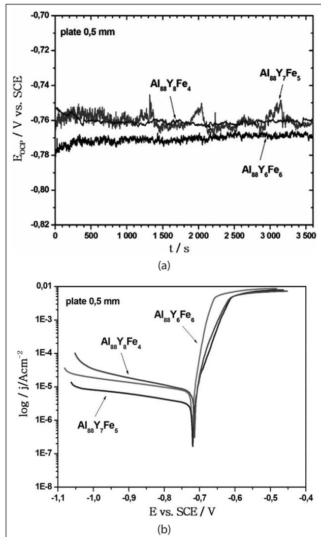
**Figure 2** Variation of the open-circuit potential with time (a) and polarization curves (b) in 3,5 % NaCl solution at 25 °C of  $\text{Al}_{88}\text{Y}_{8-x}\text{Fe}_{4+x}$  ( $x = 0, 1, 2$  at. %) alloys
