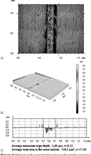
**Figure 5** Optical and axonometric views of sample wear track (a, b) and the wear profile on transverse crosssection (c) after the dry sliding of Ti13Nb13Zr—Al<sub>2</sub>O<sub>3</sub> friction pair.
