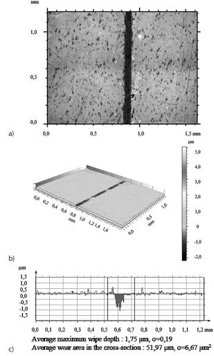
Figure 7 Optical and axonometric views of sample wear track (a ,b) and the wear profile on transverse cross-section (c) after the dry sliding of Ti13Nb13Zr TiO<sub>2</sub>— $AI_2O_3$  friction pair.
