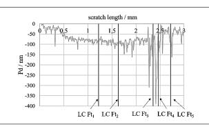
Figure 2 Scratch test results - penetration depth of the indenter (Pd)
