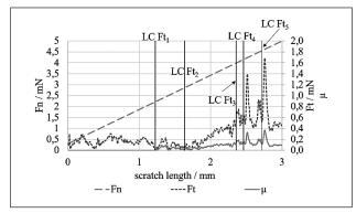
Figure 1 Scratch test results - graph of variation of loading force (Fn), coefficient of friction ( $\mu$ ), friction force (Ft)
