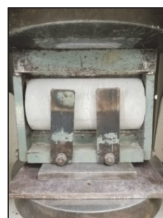
Figure 5 Splitting tensile test arrangement
