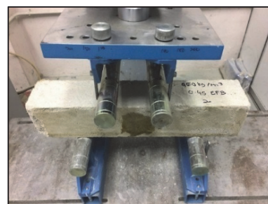
Figure 4 Bending test arrangement
