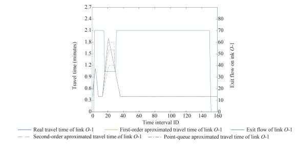
Figure 6 – Travel Times and Exit Flow Rate of the Link (O,1) with an Inflow Rate of 8000 vph
