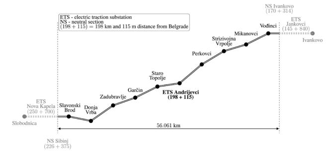
Fig. 2. Croatian Railways Corridor X section area supplied from ETS Andrijevci with the corresponding passenger stations.
