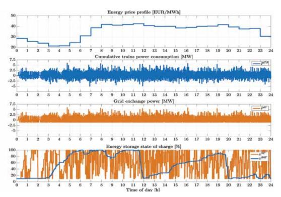
Fig. 4. Daily power flows for system operation with only higher level MPC installed and grid receptiveness of -1 MW
