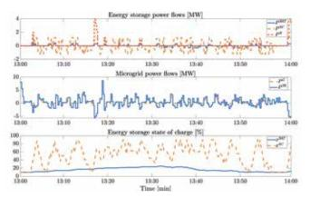
Fig. 5. One-hour system behavior without coordination.
