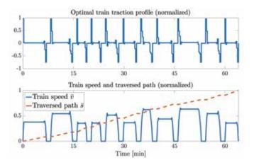
Fig. 3. Energy-optimal train traction force, speed and traversed path profiles while traveling from Slobodnica to Ivankovo.
