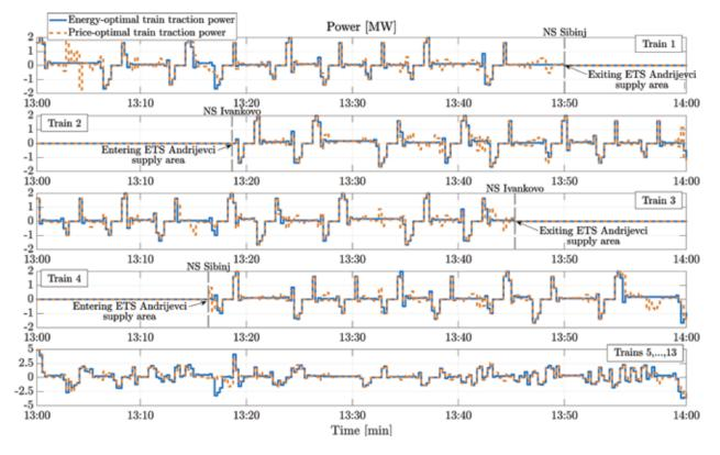
Fig. 7. Power consumption profiles of all trains supplied from ETS Andrijevci, before and after hierarchical coordination, for a one-hour system operation
