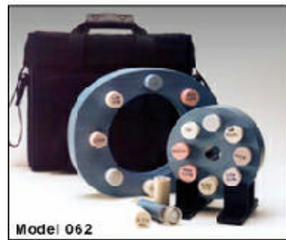
Figure IV - 25: Phantom Model 062 from CIRS compagny.
