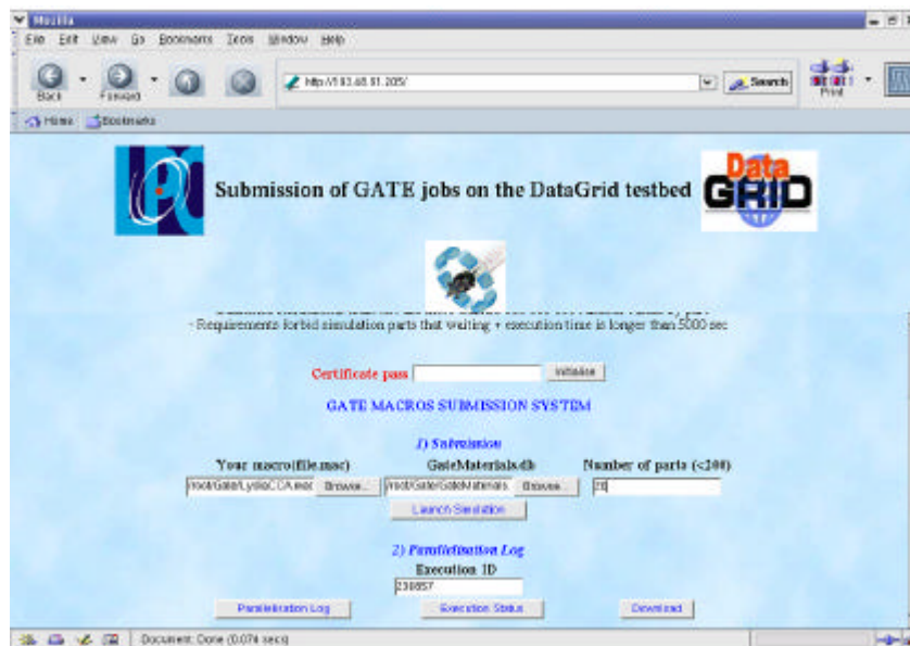
Figure V- 8: A web portal prototype for the parallelisation and submission of GATE simulations on the EDG testbed.
