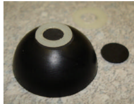
Figure I- 19: NIST WT1 solid phantom with different cap heights used for the concave ophthalmic applicators.
