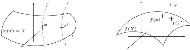
Fig. 1. Left: two points x and x' in the parameter space X . Each dotted “curve” represents a set of points where the function f is constant. Each one is a variety of dimension 7 and is parameterized by the group of similarities in R^3 . In order to obtain uniqueness of the solution, we cut back the parameter space X on a shorter space implicitly defined by \{x \in X, c(x) = 0\} , and so each “curve” cuts it just in one point. Right: a point y in the measurement space Y , the image of X by f and of its points x and x' ( f(X) , f(x) and f(x') ). f is one to one between \{x \in X, c(x) = 0\} and f(X) .
