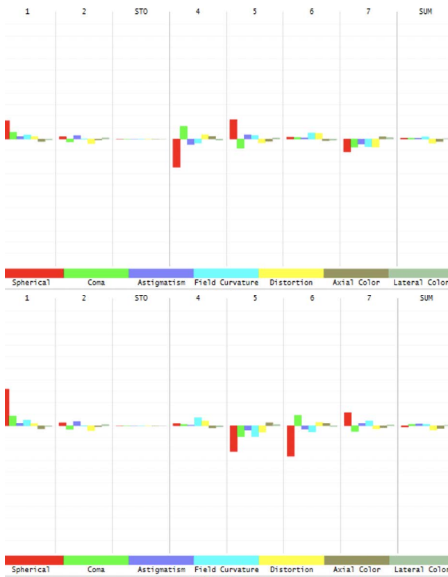
Figure 8: Seidel Diagram [8] from OpticStudio [19] indicating the main aberrations of two Cooke triplet systems: based on new solutions 1 and 84 - above and below, respectively (numbering of solutions is taken from Figure 5). Columns labeled 1, 2 and 4-7 correspond to the six lens surfaces; for each such surface the spherical, coma, astigmatism, field curvature, distortion, axial and lateral color aberrations are shown with different colours. The height of each coloured bar shows the strength of the corresponding aberration. Maximum aberration scale is 0.5[mm], horizontal grid line spacing is 0.05[mm]. Rightmost column labeled SUM shows the total aberrations of the system. Obviously, the two solutions lead to a different behaviour of the system (different amount of aberrations in each lens). Both solutions are good as indicated by low sum aberrations.
