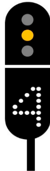
Figure 2. A yellow signal with number 4 indicating a required speed reduction to 40 km/h, to be reached by the next signal.
