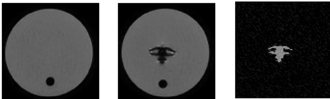
Fig. 5. Schematic showing the processing steps involved in quantifying the artifact size. (left) Reference image acquired with the nylon rod present as a black hole. (centre) Image acquired with implant in place. (right) After correction for any slight positional changes and intensity normalization, the pixels showing > 30\% change in intensity are displayed, and summed to give the total number of pixels which constitute the artifact size.
