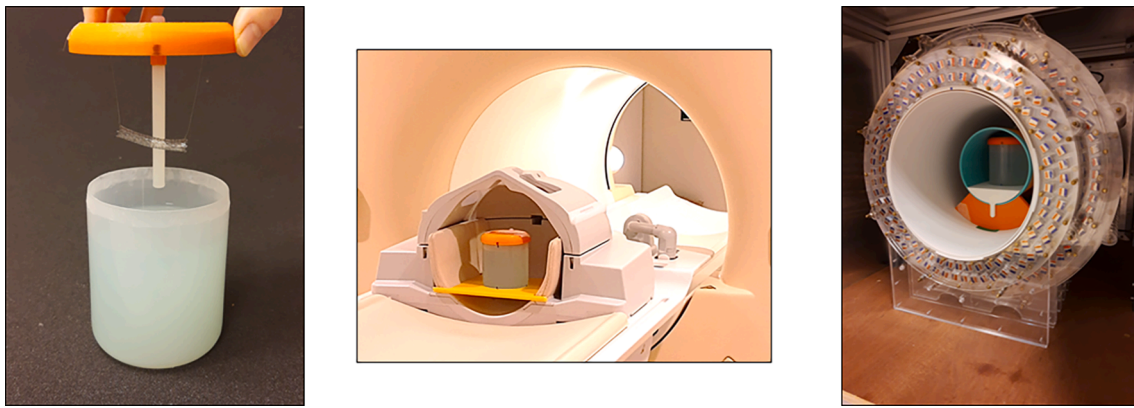
Fig. 4. (left) Photograph of the set up used for measurement of image artifacts. A cylindrical container is filled with \text{CuSO}_4 doped water. The lid integrates a solid nylon rod and the particular device is attached using thin nylon string, and located in the centre of the cylinder. A 3D printed former was designed to locate the phantom in the centre of the magnet for reproducible positioning. (centre) and (right) illustrations of the physical set up on the 3 T and 50 mT systems, respectively.
