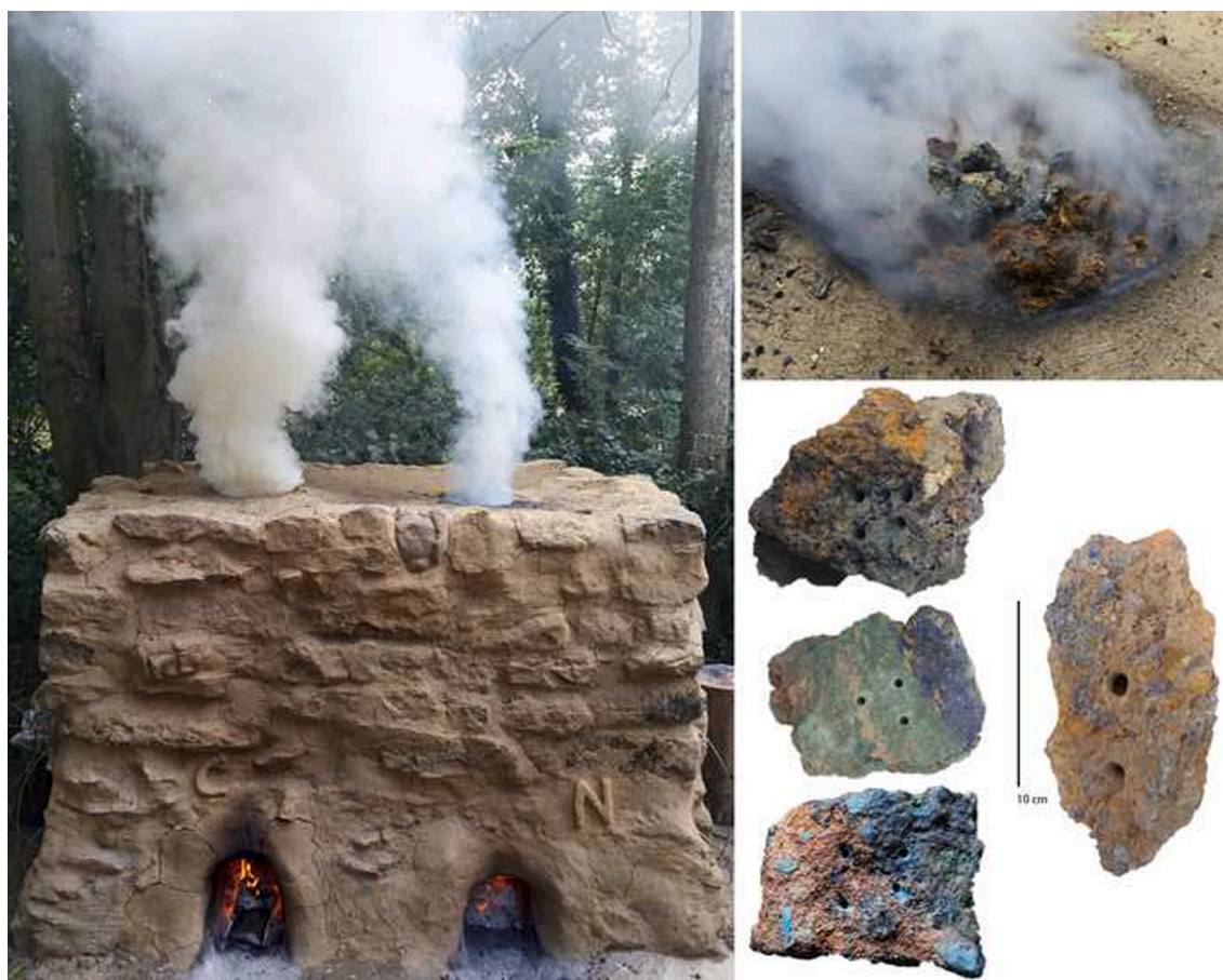
Fig. 2. Experimental furnaces at Aubechies: C for green wood, N for charcoal - Blocks of copper carbonate ore (from Morocco) – Loading the column with green wood blocks, fresh donkey dung and ore blocks © Georges Verly. (For interpretation of the references to colour in this figure legend, the reader is referred to the web version of this article.)
