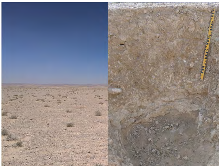
FIGURE 5 Current state of the ancient field and \text{CaCO}_3 accumulations (calcic horizon) in the soil profile. Numbers in the ruler indicate 10, 20, 30, 40 and 50 cm [Color figure can be viewed at wileyonlinelibrary.com ]
