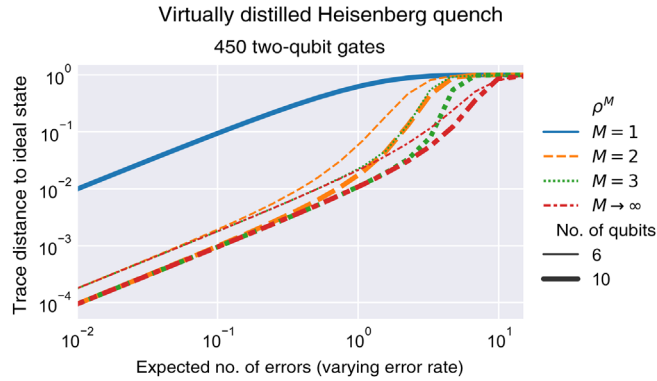
FIG. 8. The error in the unmitigated noisy states ( M = 1 ), the states accessed by virtual distillation ( M = 2, 3 ), and the dominant eigenvectors of the density matrices ( M \rightarrow \infty ), for states generated by the Trotterized time evolution of a Heisenberg model. We plot the trace distance to the state obtained from noiseless evolution as a function of the expected number of single-qubit depolarizing errors. The expected number of errors is varied by changing the error rate per gate, fixing the number of two-qubit gates to be 450. We show these data for six- and ten-qubit systems (differentiated by the size of the markers). As we increase the system size from six qubits to ten, we observe that the error (quantified by the trace distance to the ideal state) decreases for the error-mitigated states ( M > 1 ).
