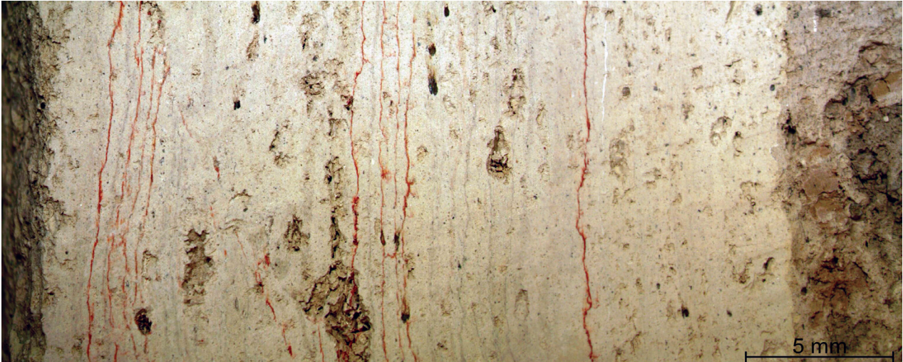
Figure 16.9. Microscopic image of a multi-layered plaster from B.17; the consecutive marl layers are observable separated by red pigment or by soot (photograph by Gesualdo Busacca).
