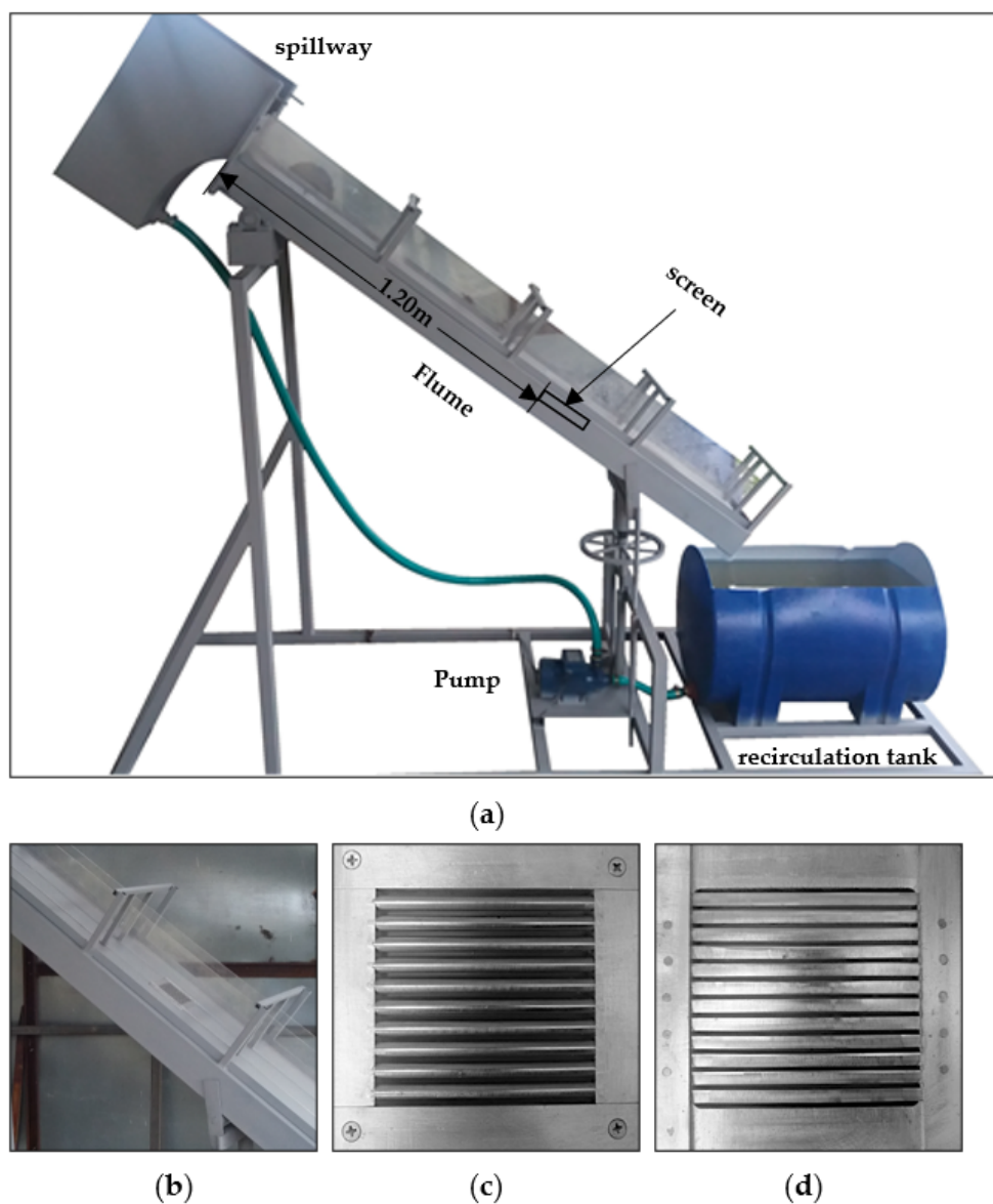
Figure 2. (a) Variable-slope screen testing flume; (b) screen installed in the test flume; (c) test screen triangular wire (d) test screen circular wire.
