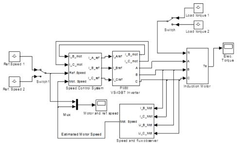
Figure 2. Simulink model of sensorlees speed control system of induction motor
