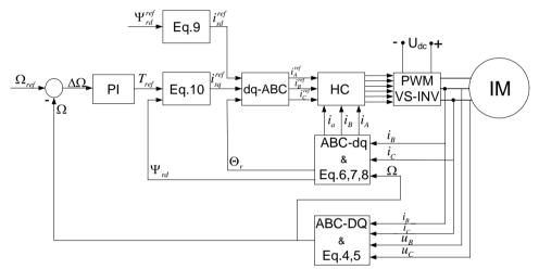
Figure 1. Sensorlees speed rotor flux oriented control system of induction motor
