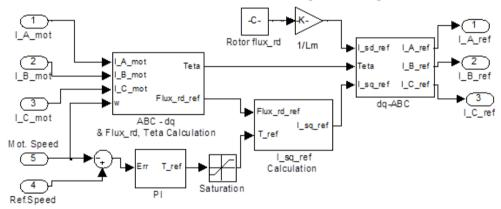
Figure 3. Simulink speed control system
