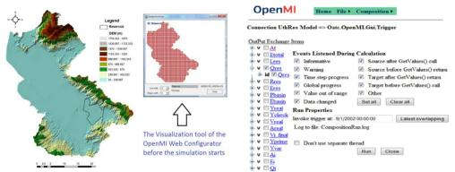
Fig. 5 Left) Digital Elevation Model of Lake Karla watershed in the location of the reservoir and visual representation of the model grid cells in the Web Configurator. Right) Variability of input/output exchange items in the linked simulation and monitoring of process interrupts
