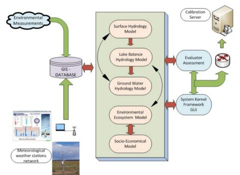
Fig. 2 The architecture of the collaborative modelling framework.
