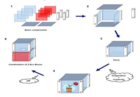
Fig. 4. The procedure of Eco-Box assemblage shows subsequently and it can combine two boxes together.
