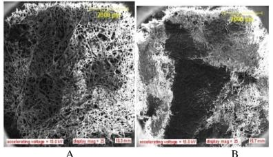
Plate 1 – SEM cross-section images of (A) Corn husk (B) Plantain stalk (Magnification 25x)
