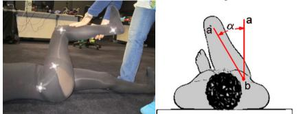
Fig. 4. To measure the adduction, the leg was positioned toward the centre of the body
