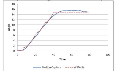
Figure 9: Example of the adduction angle in terms of time for the MoCap and Wiimote
