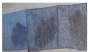
Figure 15. Photographic view of chlorine bleached samples after water repellency test
