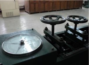
Figure 1. Horizontal tensile strength tester
