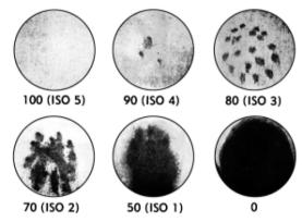
Figure 13. Standard Spray test ratings according to AATCC 22-2005
