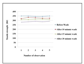
Figure 2. Graphical presentation of tensile strength (lbf) in warp way
