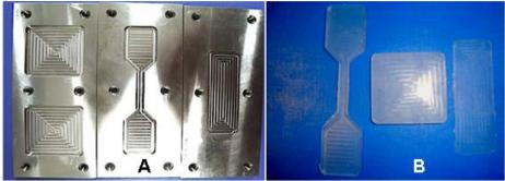
Figure 4: Control specimens (SP) and mould, A- Stainless steel moulds designed according to ASTM specifications for production of tensile, tear, hardness and percentage elengation test, B- SP (Sil-25) specimens for tensile, tear, hardness and elongation testing.
