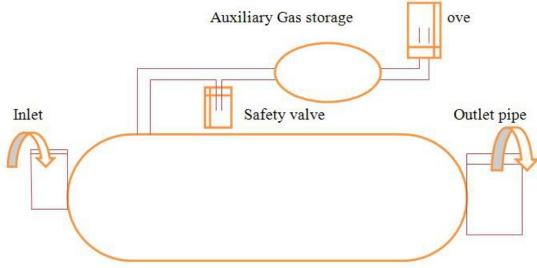
Figure 2:An Idial Biogas Plant
