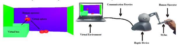
ii) Navigation in a virtual pipe with changes in the geometric characteristics (verification of position, velocity, collisions and runtime): the user attempts to resolve the virtual tube without contact or collision. The tube can be modified dimensions. Position, velocity, collisions and run time are evaluated.
