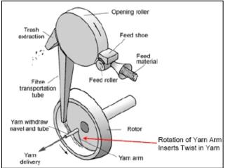
Fig. 02: Principle of Rotor spinning (Sheikh & Emeritus, 2013)
