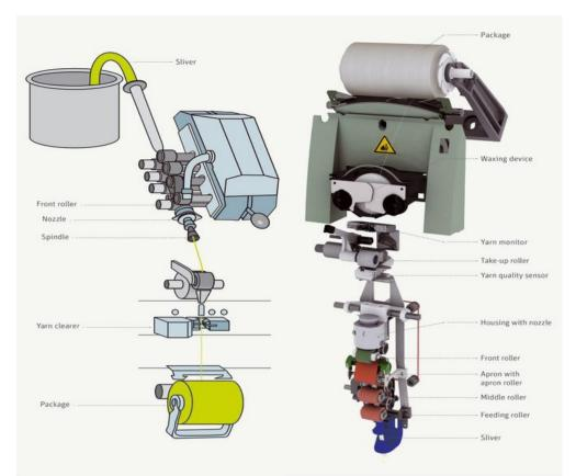
Fig 04: Air-jet spinning principle by Murata (MVS) (left) & by Rieter (J 10) (right)
