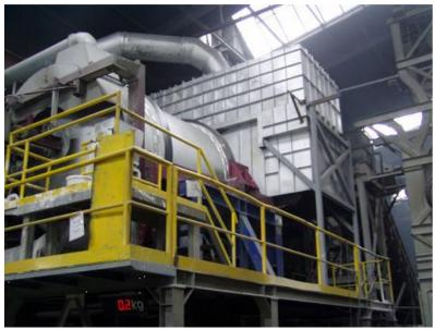
Fig. 1 10 ton – low salt rotary furnace
