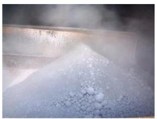
Fig. 5 First experiments with liquid binders, partially disintegrated pellets
