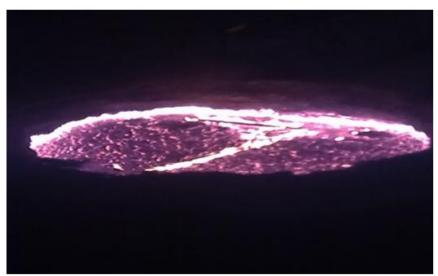
Fig. 12 Finished lower blow, slag has the appearance of a typical synthetic slag
