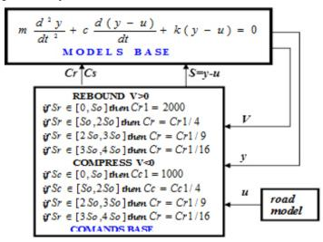
Fig 7 VZN based Suspension system, <sup>1</sup>/<sub>4</sub> car 1Degree, multi-model
