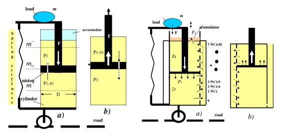
frame (ie. piston rod) called stroke S = y-u. The arch of suspension develops an elastic force Fs = kS (where k is the coefficient the elasticity of the arch)
