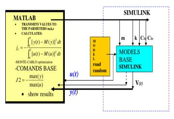
Comparison with DSA suspension provided with suspension system features a shock-absorber VZN was done by comparing the degree expressed by new two performance indicators  $J_1$  and  $J_2$ . Indicator  $J_1$  is expressed as the ratio of the variance of the output signal y of the suspension and variance of input signal u:
