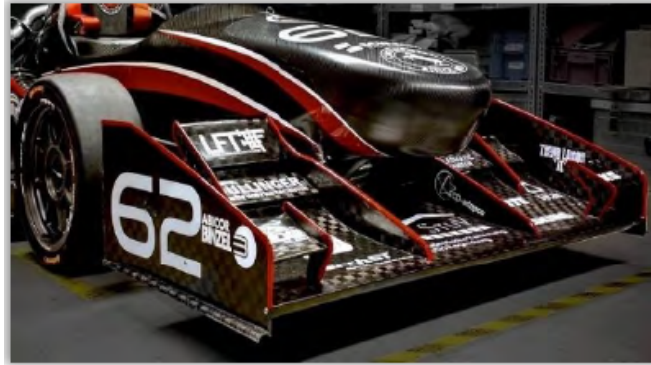
Figure 2.3: Typical FSAE car front wing [4].
