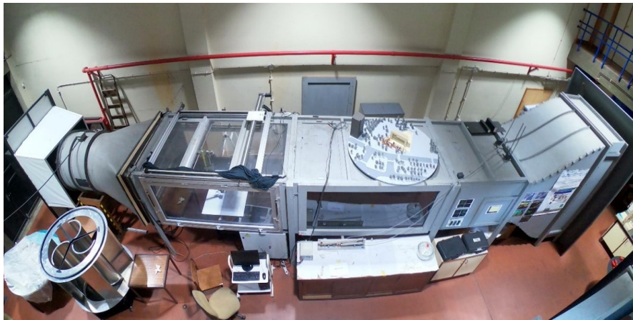
Figure 5.1: Wind tunnel used for the experiments
