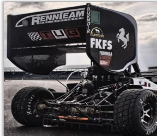
Figure 2.5: Typical FSAE car rear wing [4].
