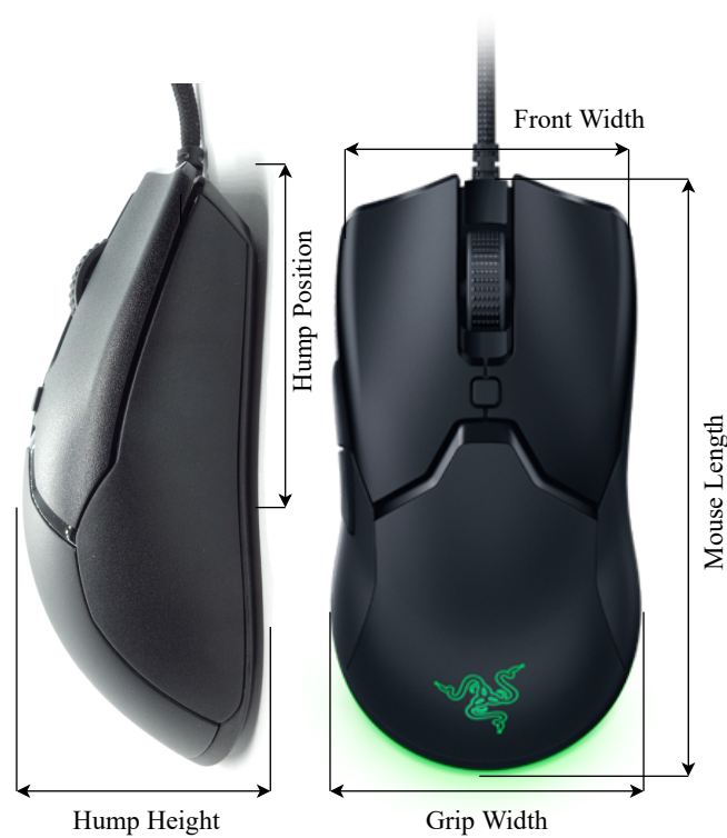
Figure 3.4: Relevant variables used in mouse design [Razer 2021].
