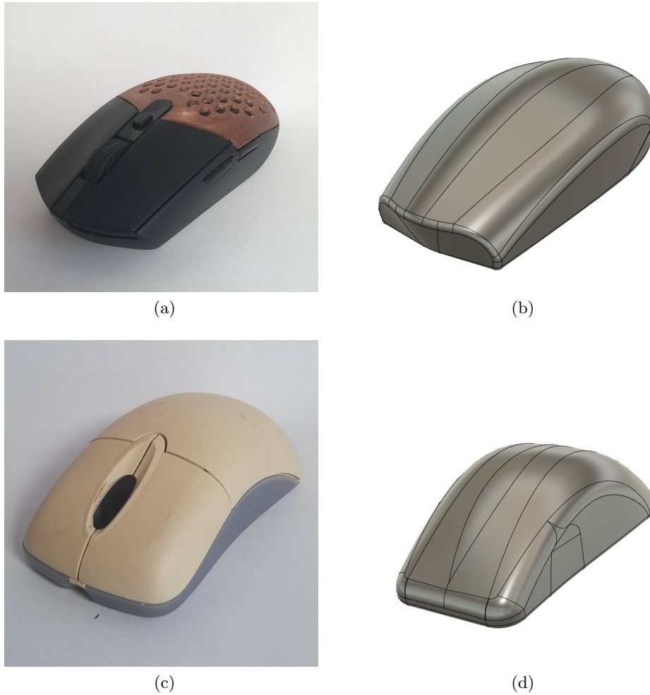
Figure 4.2: Creation of mice replicas and comparisons to the real mice: (a) Logitech G305 ; (b) Logitech G305 replica; (c) Microsoft WMO 1.1 ; (d) Microsoft WMO 1.1 replica
