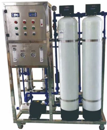
Figure 6.7: RO system water treatment, (Jiangmen Longning Water Purification Technology Co, 2021)
