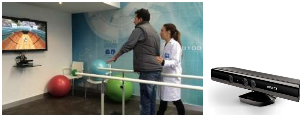
Figure 5: The Microsoft Kinect being used for rehabilitation. On the left 7 , a patient plays a rowing game. On the right 8 , the Microsoft Kinect camera that tracks the patient.
