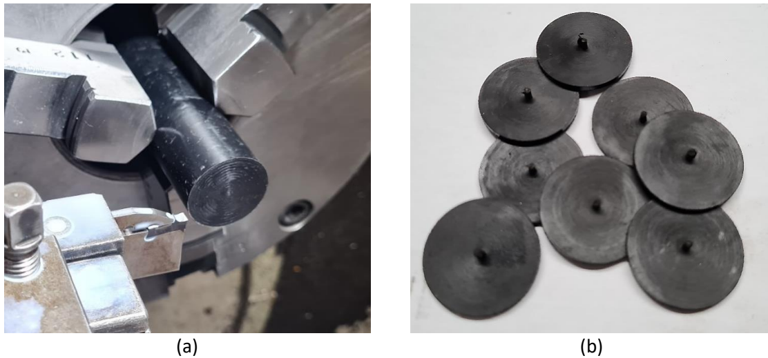
Figure 3.8 - (a) Lathing operation to turn the rods into discs and (b) ERTALON 66 GF30 discs.
