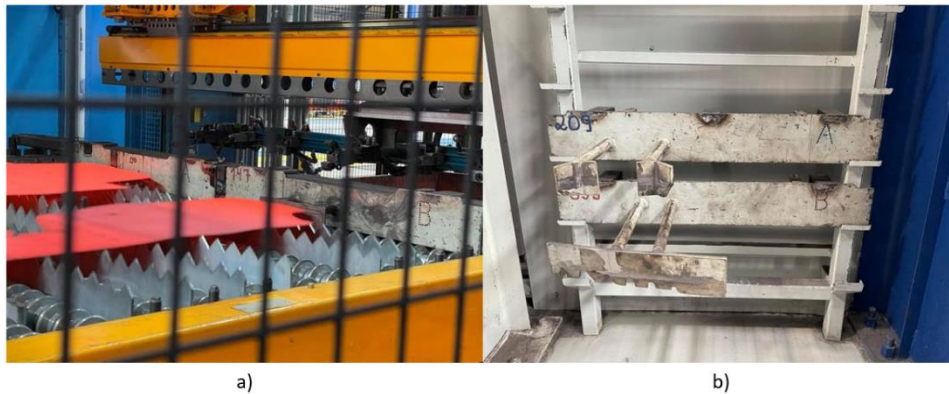
FIGURE 13: A) BLANK HITTING A STOPPER AND B) STORED STOPPERS
