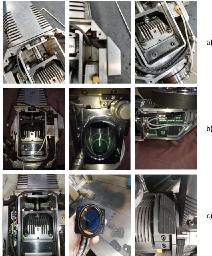
FIGURE 39: COMPARISON BETWEEN AN UNMAGNETIZED TOOL HEAD A) AND 2 MAGNETIZED TOOL HEADS B) AND C)
