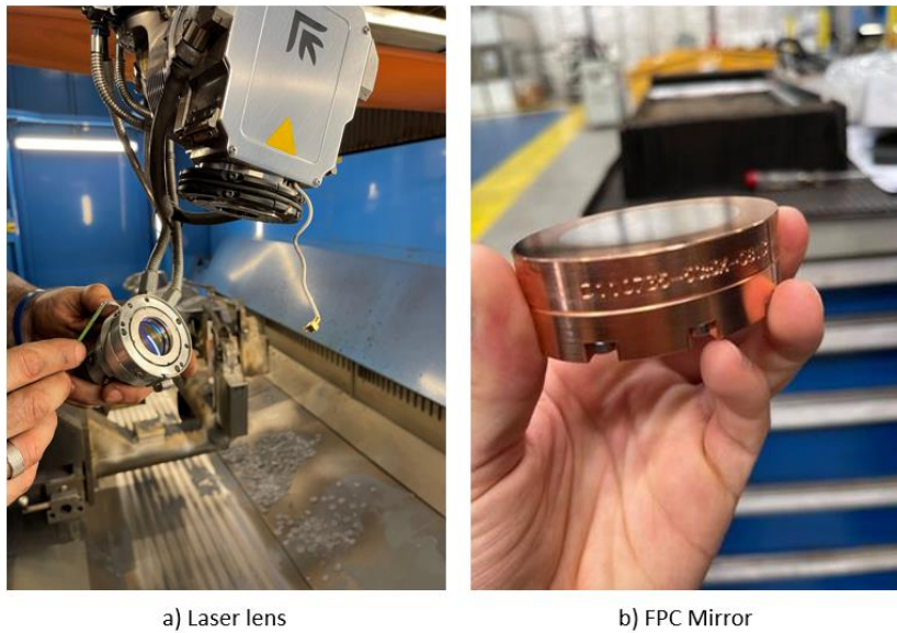
FIGURE 19: LASER TOOL HEAD COMPONENTS.
