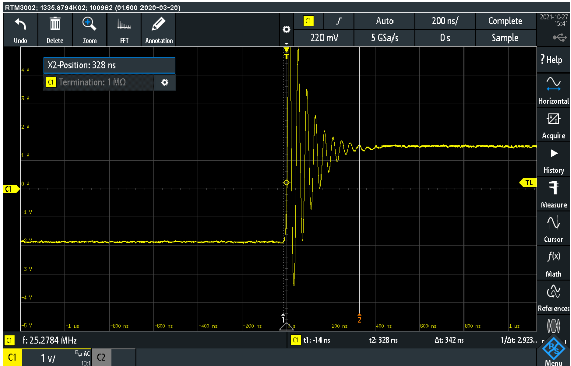
Figure 4.9: LED signal (settling time of the rising edge highlighted).
