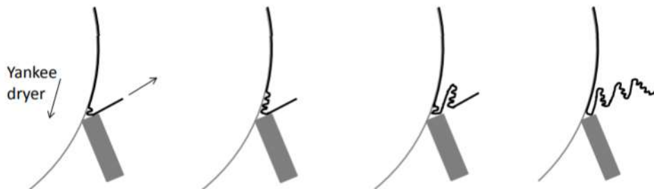
Figure 12. Creation of microfolds and macrofolds (Boudreau, 2013).
