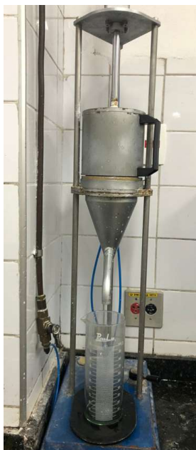
Figure 30. Schopper-Riegler apparatus with a beaker graduated of 1000 mL with direct read of the °SR.
