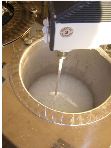
Figure 34. Tank with pulp suspension prepared
