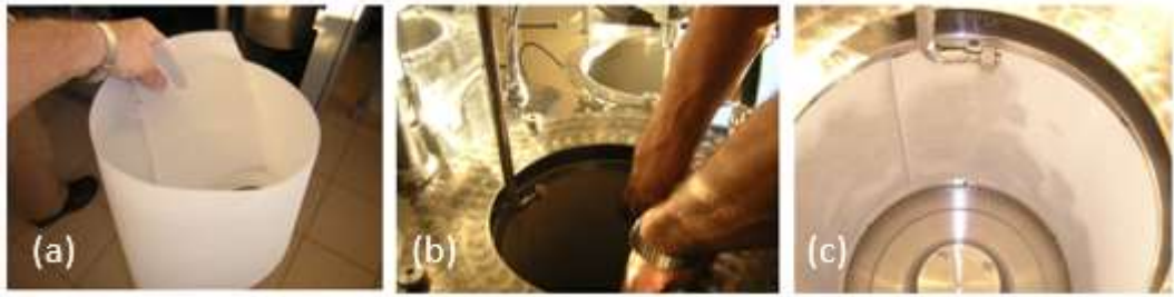
Figure 35. Wire (a), wire installation (b) and wire installed (c).
