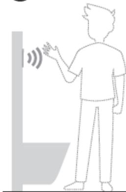
By placing the hand close to the sensor, it is possible to make complete or partial flushes.
