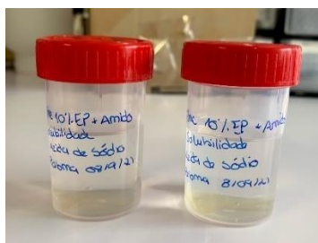
Figure 39. Film samples immersed in sodium azide aqueous solution.
