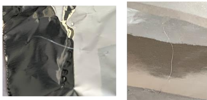
Figure 62. Electrospinning of 25% starch-based solutions prepared in 75:25 FA/H 2 O.
