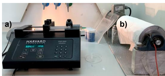
Figure 42. Electrospinning set-up used, including a) syringe pump and b) metal rotary collector with electrode wire.
