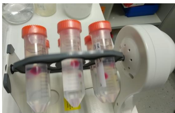
Figure 26. Apparatus used to asses agarose integrity: test tube rotator with 45 mL PBS pH 7.4 and agarose gel shape using method A2.
