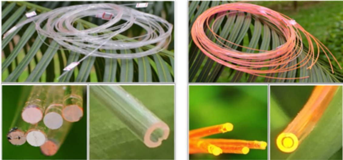
Fig. 12. Meter-scale cylindrical luminescent solar concentrators. Long-length fiber LSCs based on bulk-coated and hollow-core POFs in which the optically active layer was based on organic-inorganic hybrids doped with a \text{Eu}^{3+} -based complex and Rhodamine 6G. Adapted with permission from [28].
