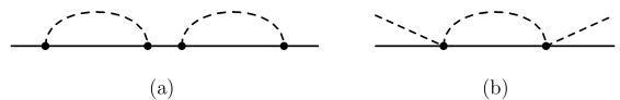
Fig. 17 Iteration of the self-energy contribution in the first order of perturbation theory (a); irreducible contribution to the bound state equation (b). Dashed lines represent pions.
