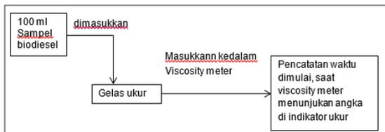
Gambar 7. Metode Uji ASTM D 455
