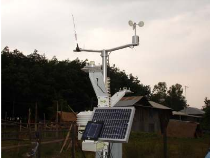
Figure 12 Local microclimate (Minimet automatic weather station, Skye Instruments Ltd, U.K.) was automatically monitored in an open field, 50 m from any trees.
