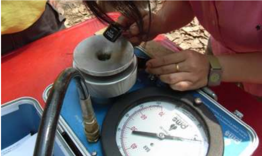
Figure 11 A Scholander type pressure chamber (PMS 1000, PMS Instrument Company, Corwallis, Oregon, USA).
