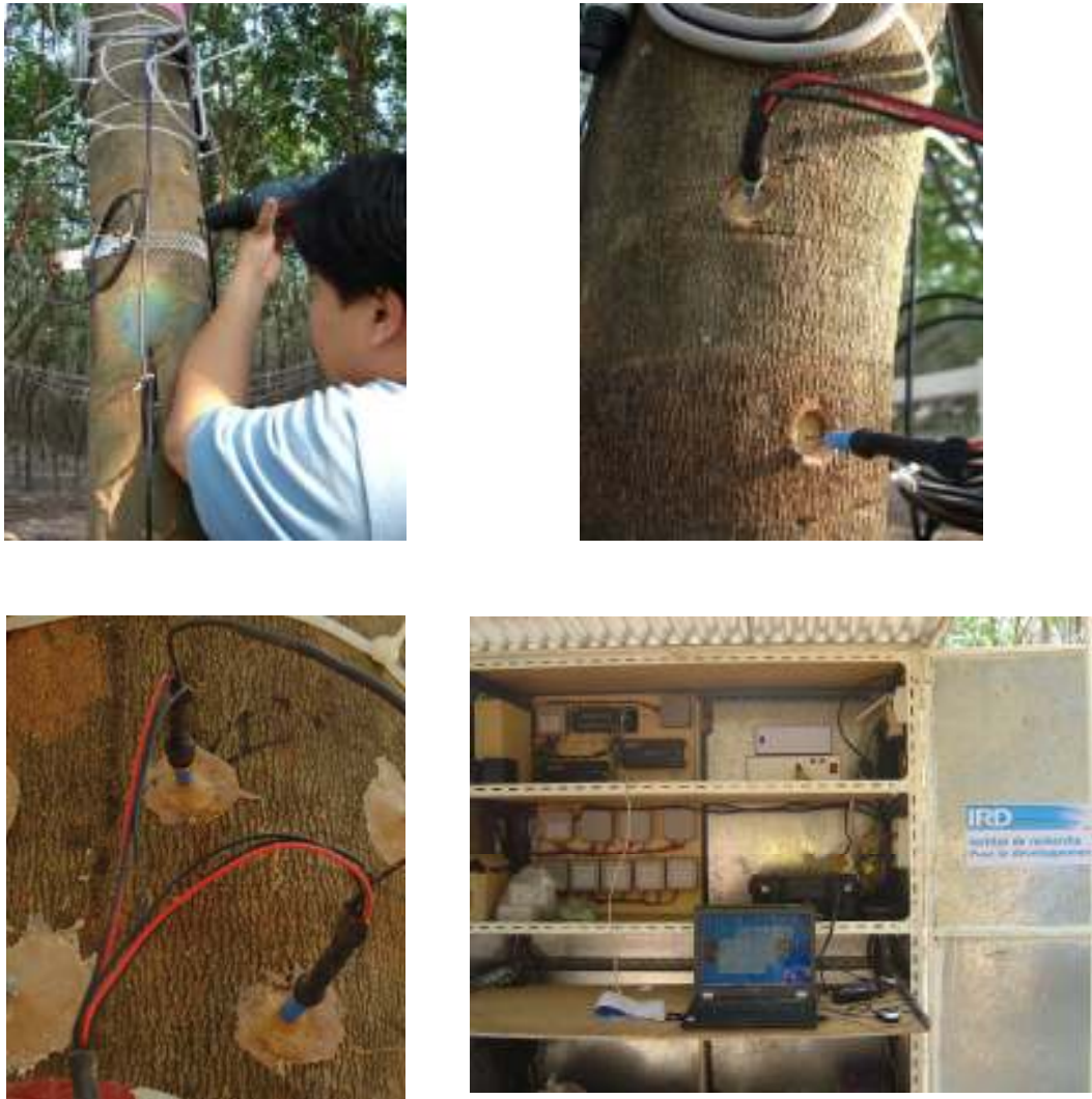
Figure 10 Installation of xylem sap flow probe in the experimental tree at a height of 1.8 m above the soil and the data logger (CR10X, Campbell Scientific, Leicester, U.K.) with multiplexer setting.
