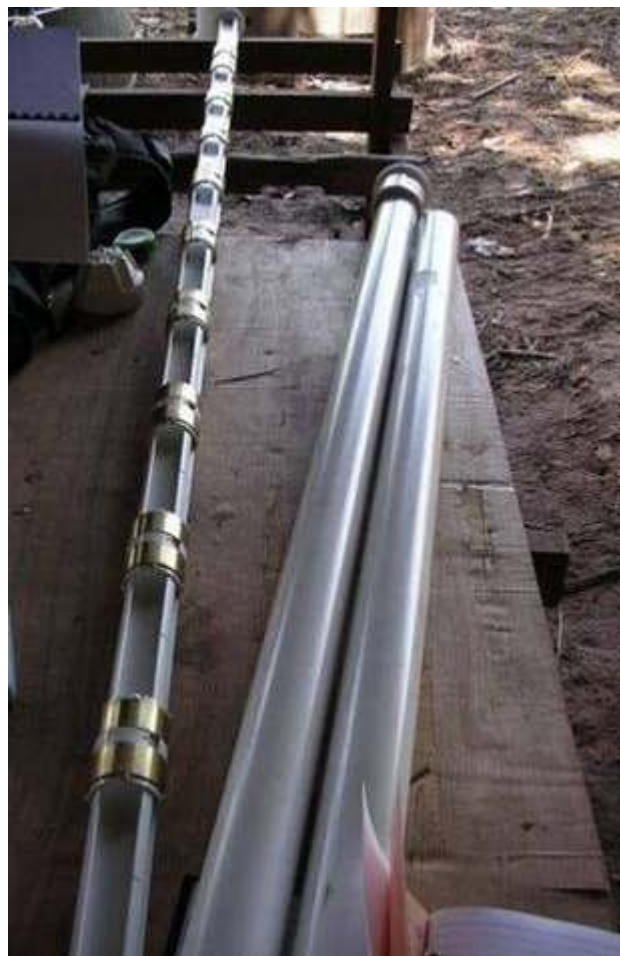
Figure 14 A capacitive probe (EnvironSCAN System, Sentek Sensor Technologies, South Australia, Australia).
