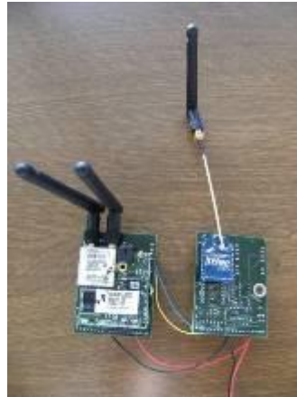
Figure IV- 4 Le multi-support WiFi-ZigBee (2 LiveNodes connectés ensemble)
