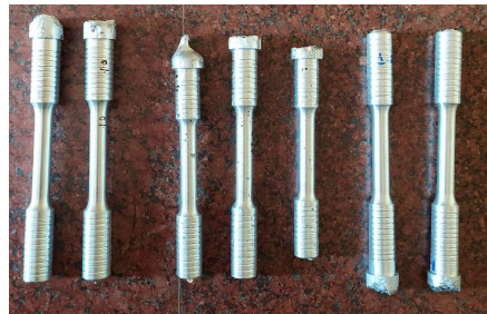
Figure 11 Specimen after machining for tensile test.
