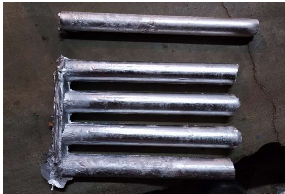
Figure 2 Casted rods after cooling.
