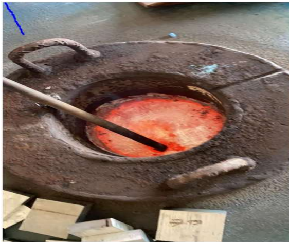
Figure 1 Molten pool of the composite in a crucible.
